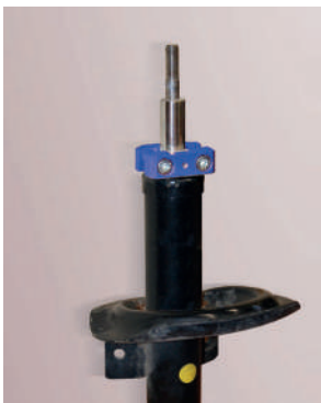
Position the clamp with the fixing screws. Do not tighten.
