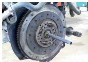
Vehicles with pilot bearing
