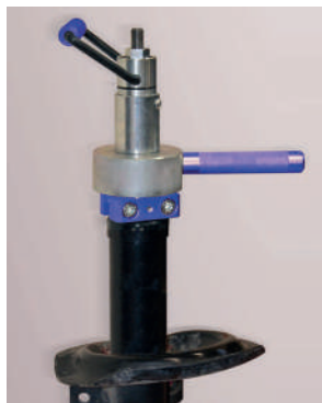
Screw the rod-puller into the support and place the shock absorber rod to the rod-puller, using the locking nut.
