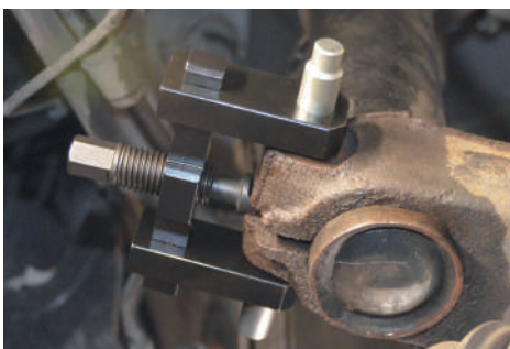
Application on shock absorber.
