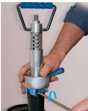
When the removal is completed, lock the clamp with the screws.
